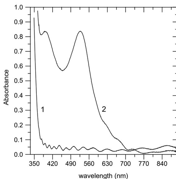
Fig. 1. Absorption spectra of the titania film with the smallest nanocrystallites (15 %wt Triton X-100): (1) pure; and (2) with adsorbed RuL<sub>2</sub>(NCS)<sub>2</sub>.
